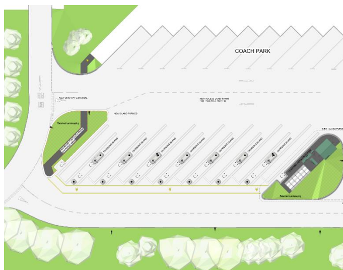
Figure 12 - Proposed charging layout at Moto Tamworth MSA, featuring drive-through bays
