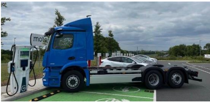
Figure 2 - HGV Tractor attempting to use a charging station designed for passenger cars
