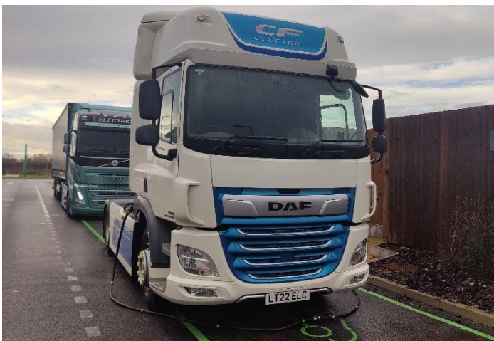
Figure 3 - Evaluating practicality of right-side charging eHGV using charger on left of bay: 7m of cable is needed
